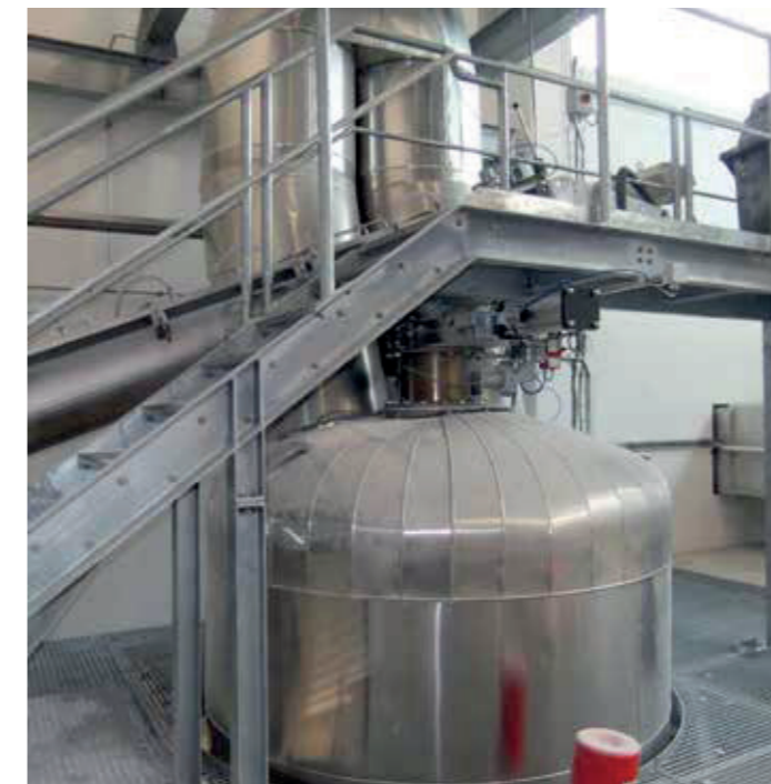
Dryer upper section with moist product infeed
