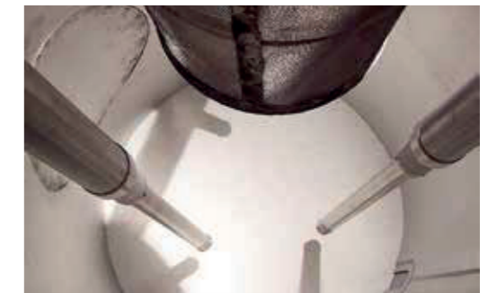
Suspension and paste dryer WS-IB-T for the creation of powders from liquids and pastes
